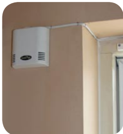
Figure 4: Spydaq sensor for monitoring air temperature & relative humidity (wirelessly) and fenestration position (wired)
