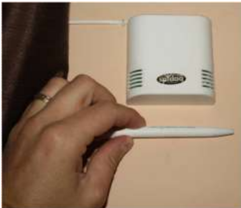
Fig. 3 Insteng sensor for recording internal air temperature, relative humidity & fenestration position
